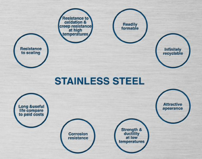
Stainless steels are a large and diverse range of engineering materials that are further developed due to corrosion resistance. The corrosion resistance of stainless steels comes from a high amount of chromium higher than 12 wt%. The greater the amount of chromium, as well as some of the elements in nickel-molybdenum-alloy, will increase the corrosion resistance properties.
